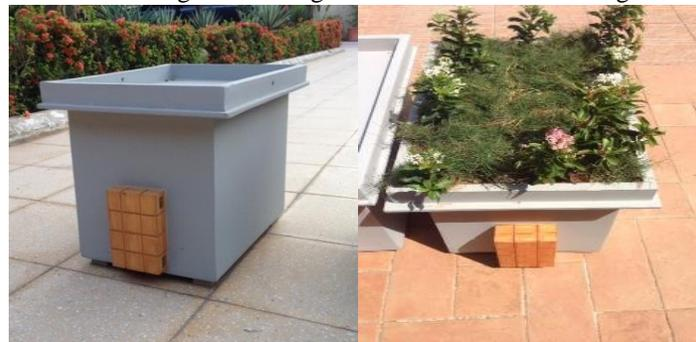
Fig. 2: The two model buildings used in the experiment (left without rooftop garden while right with rooftop garden).
